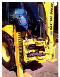
This customer also uses the KPL-24 lubricators as mobile greasing systems.
