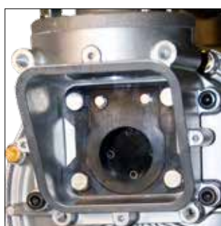
Only 4 bolts to access flap valves
