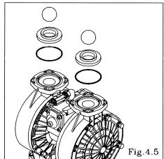
• Remove the ball, valve seat and O ring. [Fig.4.5]
