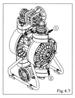
• Remove the 6 (8 on the NDP-80) retainer bolts "1" from the out manifold, and remove the protector and out manifold. [Fig. 4.7]
