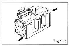
• Remove the 8 cap A and cap B retainer bolts, and remove cap A and cap B. [Fig.7.2]
