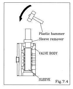
• Remove the sleeve using the sleeve remover (special tool: Part number 713180). [Fig.7.4]
