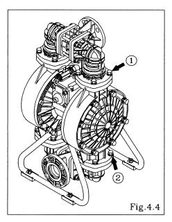
$\blacksquare$  Remove the 8 retainer bolts "1" from the out manifold, and remove the out manifold. [Fig. 4.4]
