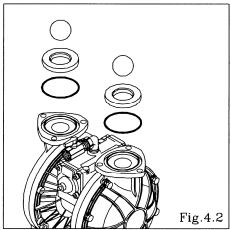
$\bullet$  Remove the ball, valve seat and O ring. [Fig.4.2]
