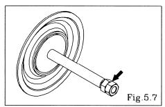
• Fix a double nut to one end of the center rod and take the diaphragm and center disk off the opposite end. [Fig.5.7] Be careful not to scratch or score the center rod.
