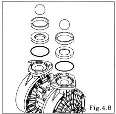
• Remove the ball, valve guide (only NDP-80), valve seat and O ring. [Fig.4.8]
