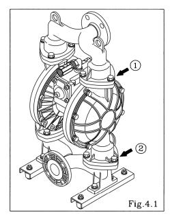
• Remove the 6 (8 on the NDP-80) retainer bolts "1" from the out manifold, and remove the out manifold. [Fig.4.1]
