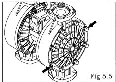
• Remove the 16 (24 on the NDP-80) retainer bolts from the out chamber, and remove the out chamber. [Fig.5.5]
