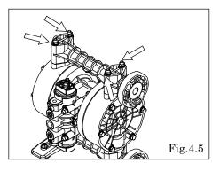
• Remove the 4 retainer nuts from the upper side of tie rods, and remove the out manifold. [Fig.4.5]
