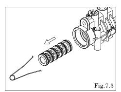
• Remove the sleeve using the sleeve remover (special tool: Part number 713148). [Fig.7.3]
