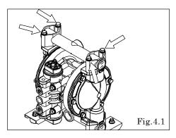
• Remove the 4 retainer bolts from the out manifold, and remove the out manifold. [Fig.4.1]
