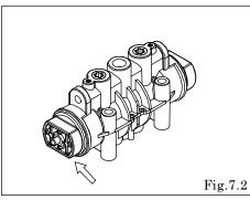
• Remove the cap A with Ajustable angle wrenches, remove packing and draw out the C spool valve assembly. [Fig.7.2]
