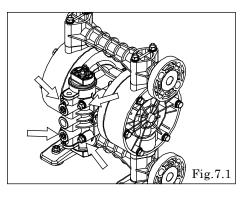
• Remove the 4 retainer bolts from the valve body, and remove the valve body and gasket. [Fig.7.1]
