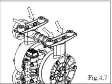
• Pull out the tie rod, and remove the base and in manifold. [Fig.4.7]
