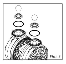
• Remove the ball, valve seat and O ring. [Fig.4.2]
