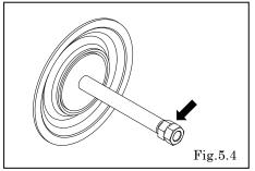
• Fix a double nut to one end of the center rod and take the diaphragm and center disk off the opposite end. [Fig.5.4] Be careful not to scratch or score the center rod.
