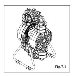
$\blacksquare$  Remove the 4 cap A and cap B retainer bolts, and remove cap A and cap B. [Fig.7.1]
