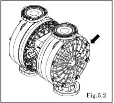
• Unscrew 16 bolts (include 8 bolts mentioned above) from the out chamber and remove the out chamber.[Fig.5.2]
