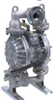
The Yamada 2:1 high pressure pump was specifically de -signed for applications where 100 PSI maximum pump operating pressure is not enough to overcome system requirements. The flow rate is roughly half of the same size pump output, though a discharge pressure of 200 PSI can be achieved with only 100 PSI air inlet pressure supplied. The 2:1 discharge pressure ratio is achieved by utilizing twice the surface area (driving both diaphragms) to double the output.
