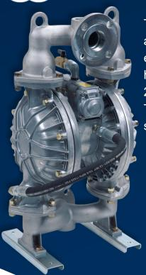
The Yamada 2:1 High Pressure pump was specifically designed for applications where 100 PSI maximum pump operating pressure is not enough to overcome system requirements. The flow rate is roughly half of the same size pump output, though a discharge pressure of 200PSI can be achieved with only 100 PSI air inlet pressure supplied. The 2:1 discharge pressure ratio is achieved by utilizing twice the surface area (driving both diaphragms) to double the output.
